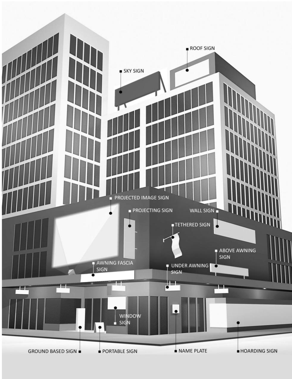
Figure 3 – Illustration of Various Signs Types
