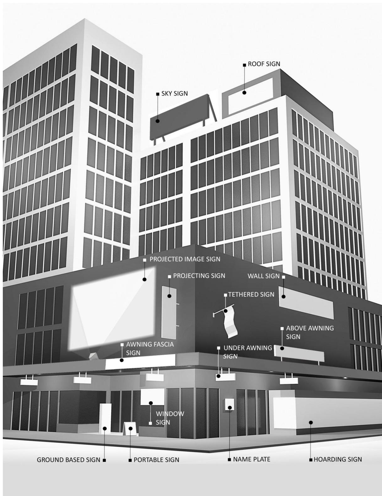
Figure 1 - Illustration of Various Sign Types.
