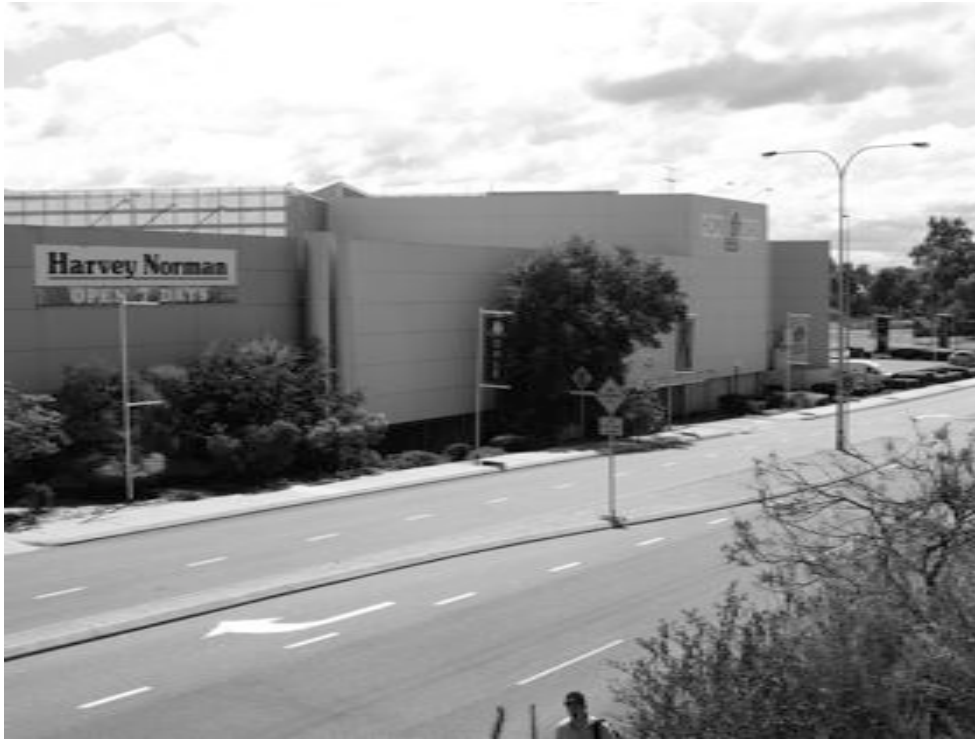
Blank walls and an under-croft car park interface with a street are unacceptable urban design outcomes.
